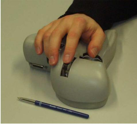
**Fig. 2.** Picture that shows the way to put the hand on the DigiHaptic.
